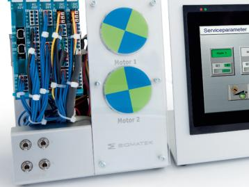
We transfered the modularity of our complete automation solution to the SSK 002-1 starter kit: It consists of the basic control unit TSY 021 in combination with an HMI and motion expansion. You can also order the units individually based on requirements.
