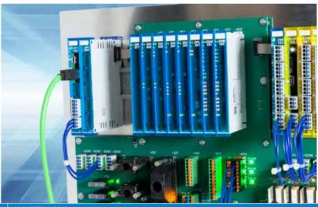
X-DIAS minimizes wiring within the machine, reduces wiring mistakes, cuts installation time and saves overall expenses.
