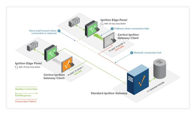
**Hub-and-Spoke with Local Client Fallback:** Use Edge Panel to add local client fallback to a hub-and-spoke architecture. Edge Panel provides visualization at the edge, a 35 day data buffer to cache PLC data while a network connection is down, and store and forward functionality for when the connection is restored.
