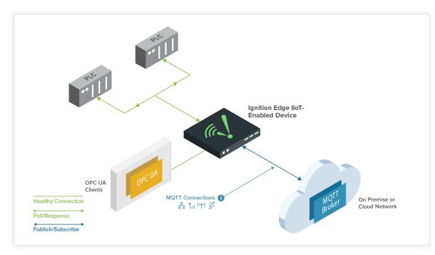
**Ignition Edge IIoT Standalone:** Use Edge IIoT as a standalone edge gateway to publish device data from the edge of the network to an MQTT broker.
