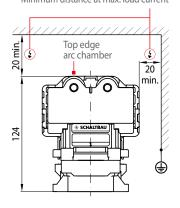
For the C310K/150, C310K/300 and C310K/500 series there is a minimum distance of 20 mm to magnetically active, live or earthed parts.
