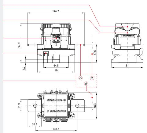
Arc chamber cover Reduces the distance to live, metallic or grounded parts
