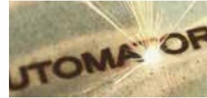
OXIDATION Dark marking on metal.
