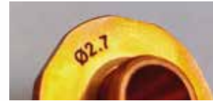
ANNEALING Dark zero-touch marking.
