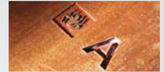
DEEP MARKING Engraving by pulverization of the material to the required depth.
