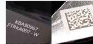
WHITENING / CLEANING / CLEAR MARKING A shallow laser marking.
