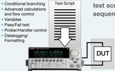
To provide the throughput demanded by production applications, embedded test scripts can be uploaded into the SMU, enabling them to run complex test sequences without computer control or communications slowing things down.
